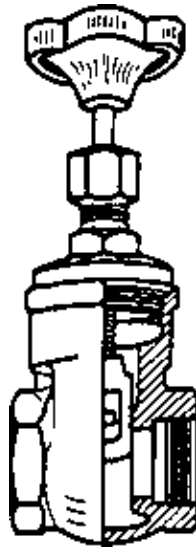
Fig. 13.6. Slide valve (half section)
